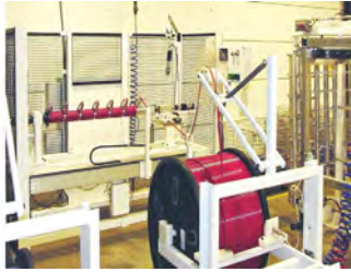
Tubing spools are used to create individual coiled assemblies.
