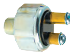
422710 STOP LAMP SWITCH NORMALLY OFF SPST OPERATES 60-120 PSI CONTACT CLOSED AT RISING PRESSURE
